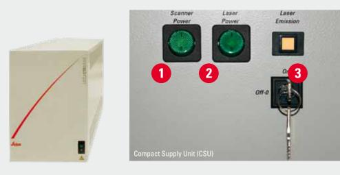
For system configuration with CSU: Turn on the ---Turn on the PC and await the booting microscope process. Then turn on the power supply control box. for the scanner 1 and the lasers 2 by pushing the green buttons and turn the
