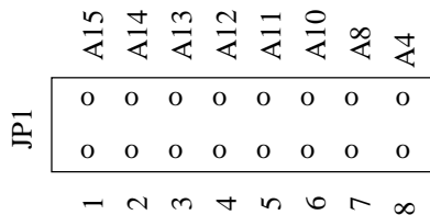
Figure 3. Jumper block JP1 address configuration.
