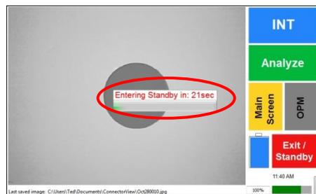
To manually place in ViewConn Pro in Standby touch the red [Exit] button on the Main Screen or Quick View Screen, then the yellow [Standby] button on the Closing Screen.
