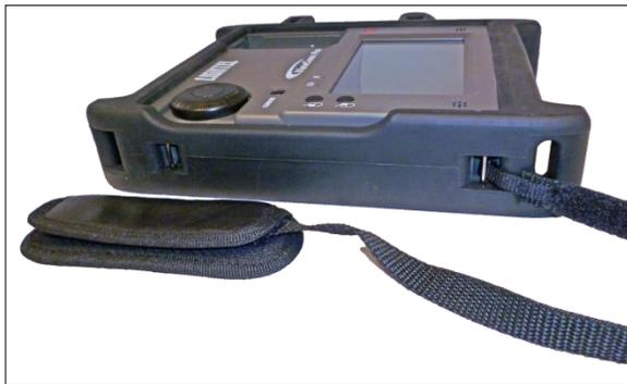
**Replace the wrist strap** – With the leather side of the strap facing away from ViewConn Pro and the open side facing toward the back, thread the loop portion of the strap under the bottom pin in an upward direction. If too difficult to grab, you may want to use tweezers or small pliers to grab the loop.
