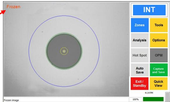
Then touch the [Capture and Save] button. The filename will be displayed in red on the screen when the file has been saved. (The red name is not displayed on the saved image.) Touch the screen again to return to the live view.
