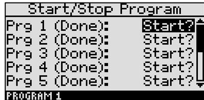
If the program is running, the Stop? option displays on the right side of the screen. To stop the program, highlight the **Stop?** option, and then press the **OK** button. The label to the right of the program number changes to “Done.”
