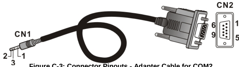
Figure C-3: Connector Pinouts - Adapter Cable for COM2
