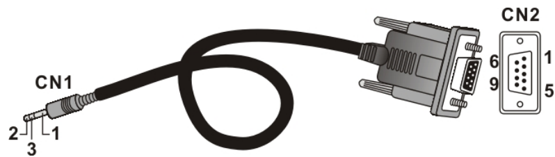
Figure C-2: Adapter Cable for COM1 - Connector Pinouts
