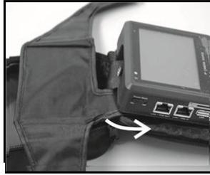
6. Fold one wing around the edge of the device, and insert the tail of the wing into the space between the device and the Velcro surface. Fasten the tail to the Velcro tightly.
