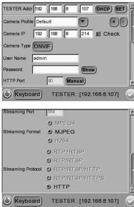
The screenshot displays two panels of the camera's configuration interface. The top panel is for general network and user settings, and the bottom panel is for streaming options.
