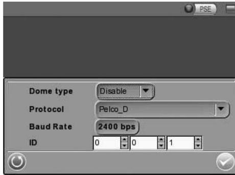
Select <Enable> from the <Dome type> drop-down list. Tap <Enter/Save>
