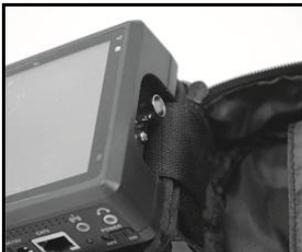
5. Lift the front part of the device up and put the sunshade's short wing into the space between the device and the self-adhesive Velcro surface. Align the wing's left edge with the left edge of the device. Fasten the short wing to the Velcro surface tightly.
