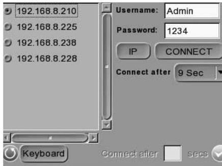
Select the target IP camera from the device list on the left top of the screen. Select the camera connection duration from the available dropdown. For a custom setting, select <Custom> from the dropdown and enter the value in the field at the bottom of the setup page. Tap <Connect> beneath the Password column to begin connecting. The live view video displays on the screen.
