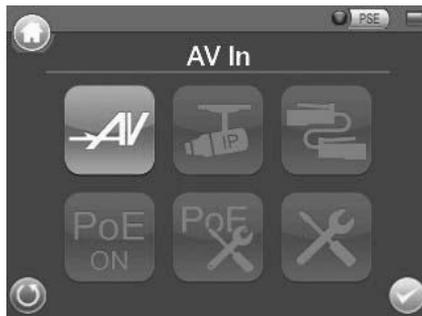
To view live video from an IP camera which supports BNC via AV In function, confirm the IP camera streaming is set as "BNC Out."
