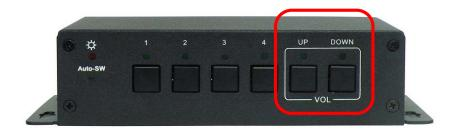
Press the button "1" for 3 seconds, the WVG4A PA will enter the auto-switching mode. The LED light of "Auto-SW" will be on. Please check the index"5.2" for the auto-switching mode. Pressing the button "1" for another 3 seconds, to quit the auto-switching and return to the regular manual switching. The LED light of "Auto-SW" will be off.
