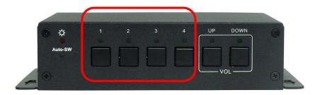
Press the buttons "Up", "Down" to control the output volume up/down. (not including the bass/treble setting)
