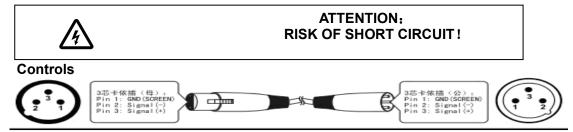
Link all DMX devices with a DMX-512 controller by using a standard,3-pin DMX cable. Connect the output of the first device with the input of the second device and the output of the second device with the input of the third device and so on.
