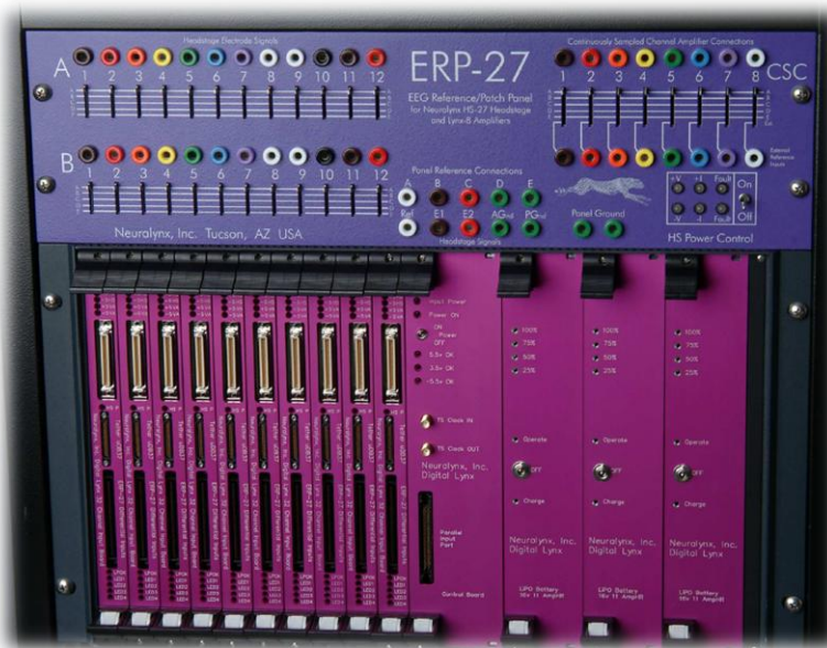
Figure 6-1 Digital Lynx in a 19" equipment rack.
