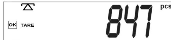
Checkweighing during Parts Counting
