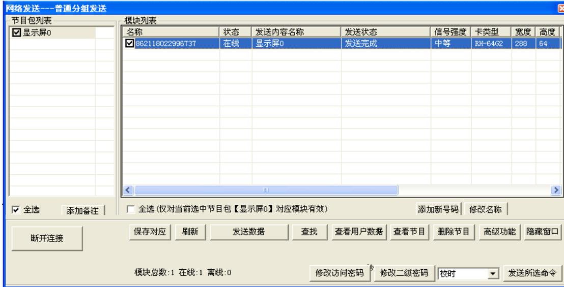
Then click "send data", After the data is sent to the display screen, the program will automatically adjust the size of typeface.
