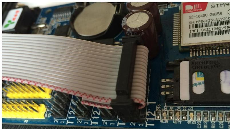
After connection above, connect the +5V terminal and GND of the 5V-power supply in indicate screen respectively with the +5V and GND of the control card, and connect the power supply, then press the test button on the control card to test whether there is error with the hardware connection, and by pressing on the test button, the display screen will be switched to a test status.
