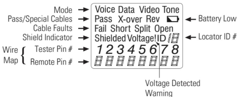
Figure 2. LCD Display Screen
