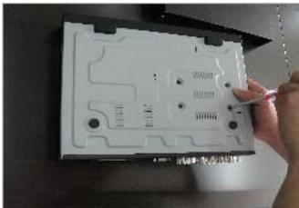
Fix the screw of hard disk sides of shell
