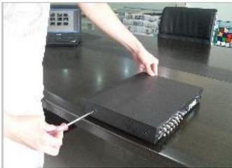
Remove the screws on both board sides of shell
