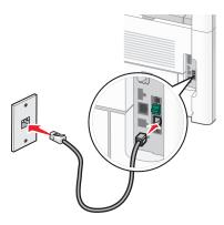
**3** Remove the protective plug from the EXT port  $\widehat{\blacksquare}$  of the printer.
