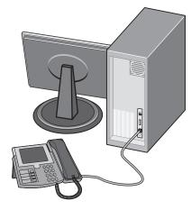
**5** Connect a third telephone cord from the computer modem to the EXT port i of the printer.
