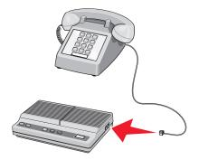
**5** Connect a third telephone cord from the answering machine to the EXT port  $\widehat{m}$  of the printer.
