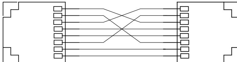
Figure A-3 Cable sequence of cross-over cable
