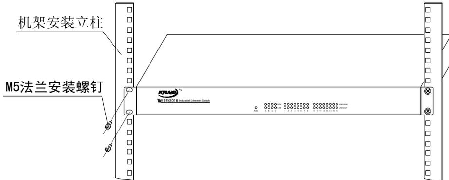
Figure 4-2 Mounting the SICOM3024 on the rack
