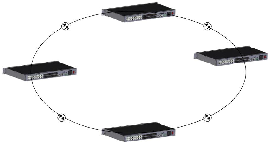
图 6-1 SICOM300 build the redundancy ring
