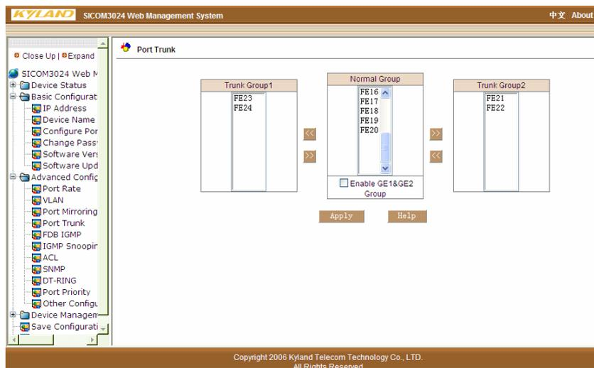
Figure 7-16 Port Aggregation Configuration
