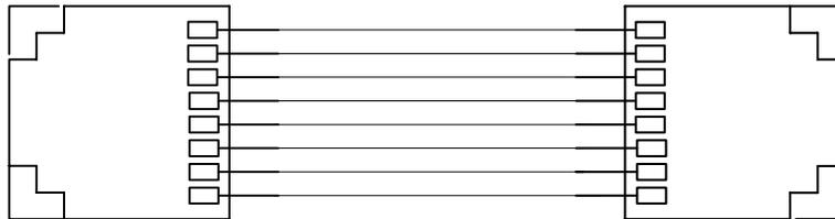
Figure A-2 Cable sequence of straight-through cable
