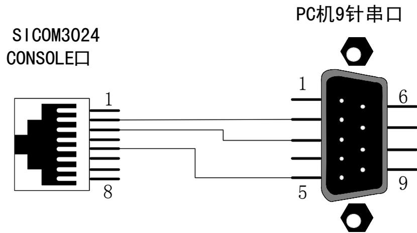
Figure 3-9 CONSOLE wiring diagram
