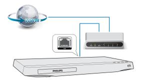
For Wi-Fi, connect a Philips Wi-Fi USB adapter (named WUB1110) to the
