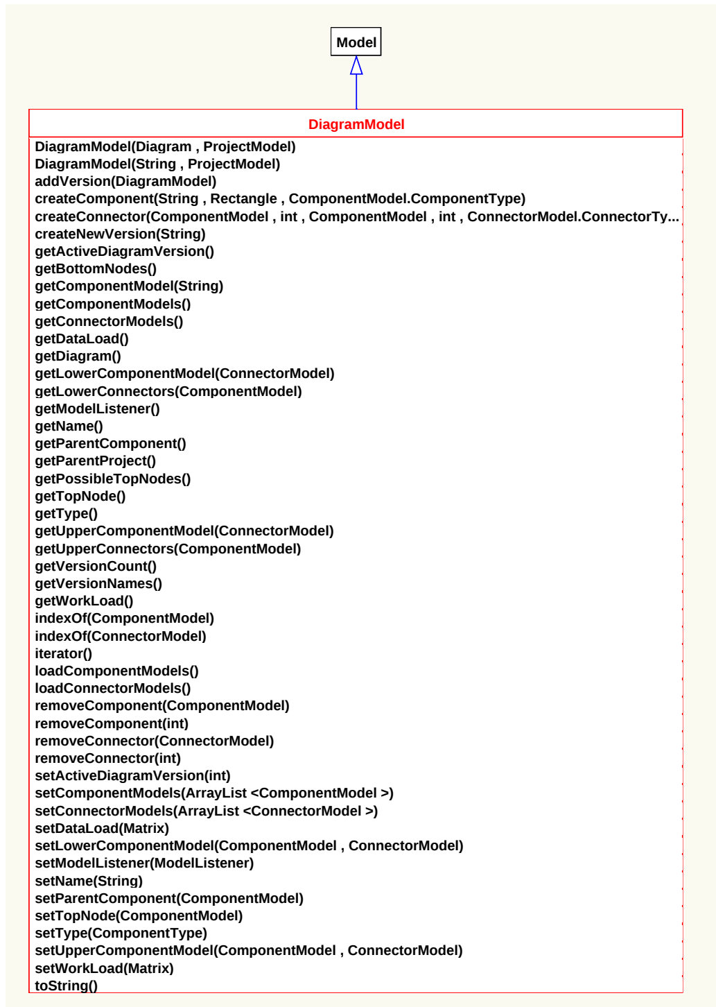
Figure 6.9: DiagramModel class diagram
