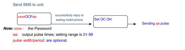
when aa=00 the SMS unit send pulse constantly
