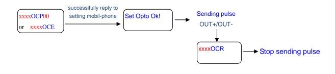
4.8 OPTO Output Port (MOSFET relay): OUT+/OUT-
