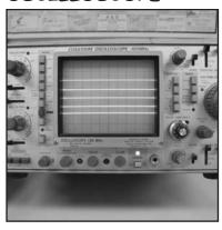
This is a powerful 100 Mhz oscilloscope with 5 channels and 12 traces. It has a four way trigger off either channels 1, 2, 3, or ALT. Trigger lock for stable automatic triggering for complex signals such as video
