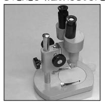
Unused stereo microscope with a large working distance and field of view. The whole microscope head can be rotated 360 degrees and can be raised and lowered on its vertical pillar. The
