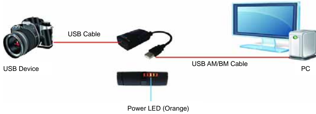
Fig 1. The USB Isolator unit is installed in-line between the PC and a connected USB device.
