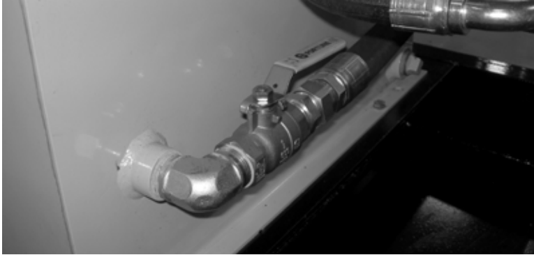
Figure 1-6. Hydraulic suction shut-off valve (shown in the open position). Turn the lever perpendicular to the fitting to shut off hydraulic oil supply to the pump.
