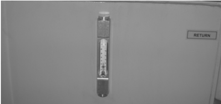
Figure 1-7. The hydraulic oil temperature/fill level gauge is on the front of the reservoir.
