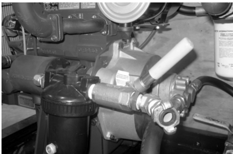
Figure 3-3. Pull the starter handle to engage the starter motor. When the engine starts, release the handle.
