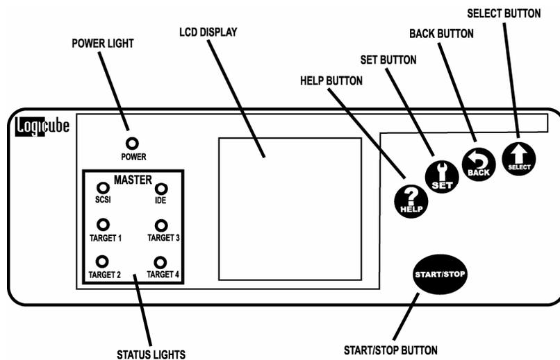
**NOTE:** The display panel will look slightly different between the OmniSCSI One-to-One™, OmniSCSI-2 and the OmniSCSI-4. Also, the Status Lights will show the number of Target drives that the unit can hold, (i.e. one Target light for the OmniSCSI One-to-One, four Target lights for the OmniSCSI-4, etc.)
