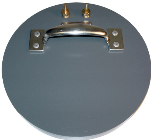
The Surface Emission Chamber
