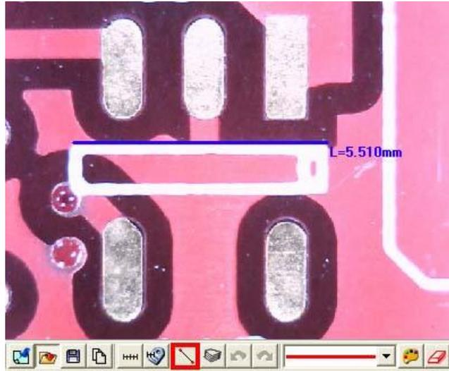
Fig.5-67 Length measurement
