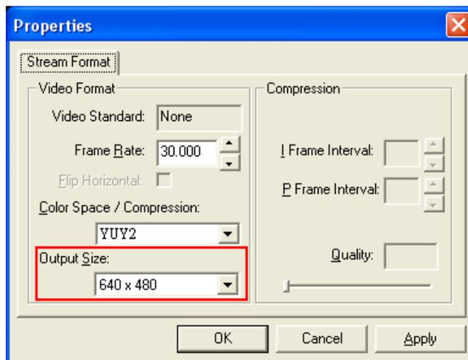
Fig.5-48 Resolution adjustment
