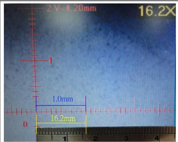
Fig 5-59 Use a metal ruler to measure the magnification.
