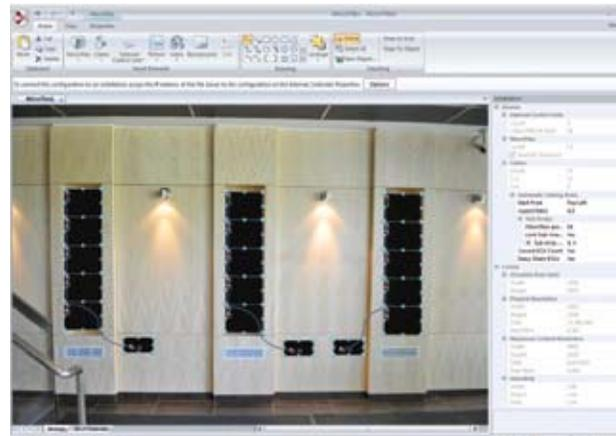
▲ Christie MicroTiles Designer tells you the energy consumption of the display, how much the total display will weigh and shows you the optimal way to wire the tiles together. All these features ensure the system you get is the system you want and the system you need.
