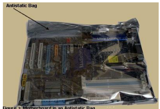
Figure 3: Motherboard in an Antistatic Bag
