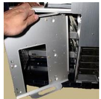
Figure 8: Remove Motherboard Tray
