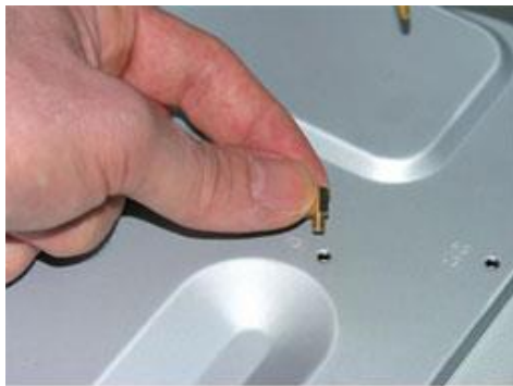
Figure 9: Screw Brass Standoffs Into the Motherboard
