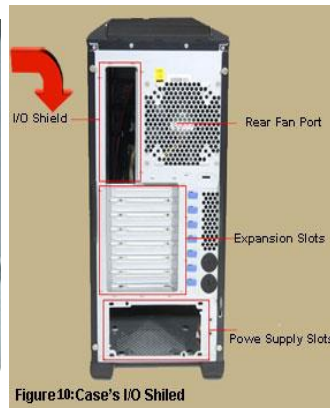
Figure 10: Case's I/O Shield
