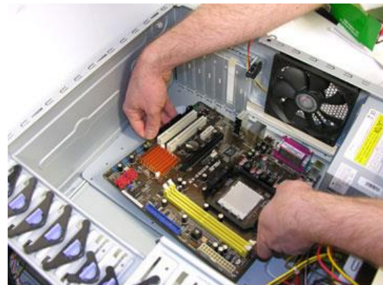
Figure 11: Mount the Motherboard
