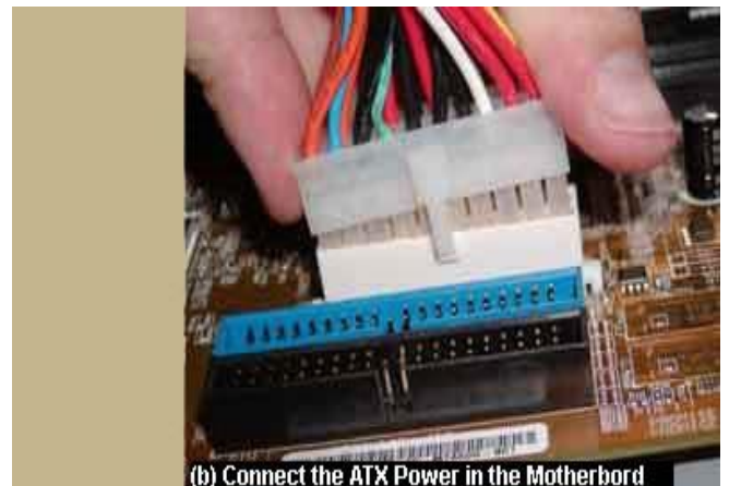
(b) Connect the ATX Power in the Motherboard
