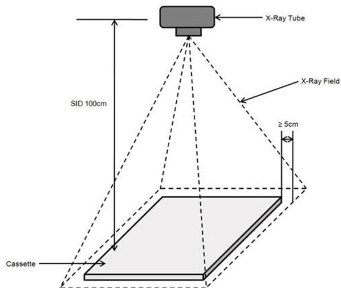
Figure 1.14. Calibration Geometry
