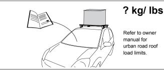
When these roof racks are to be used on a vehicle that is driven off sealed roads, the manufacturer maximum roof load rating (to be found in the vehicles User Manual) should be *divided by 1.5*. Do not forget to subtract 5kg/11lbs from your maximum carrying capacity due to the weight of the crossbars and legs.
