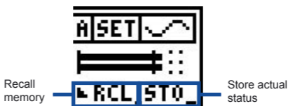
Fig 5-08, Channel status memory field
