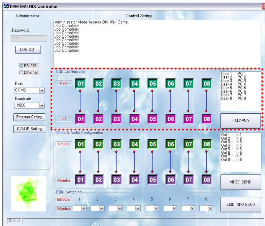
[Fig. 1-3] One-to-one switching of both Video/Audio and USB by PC program
