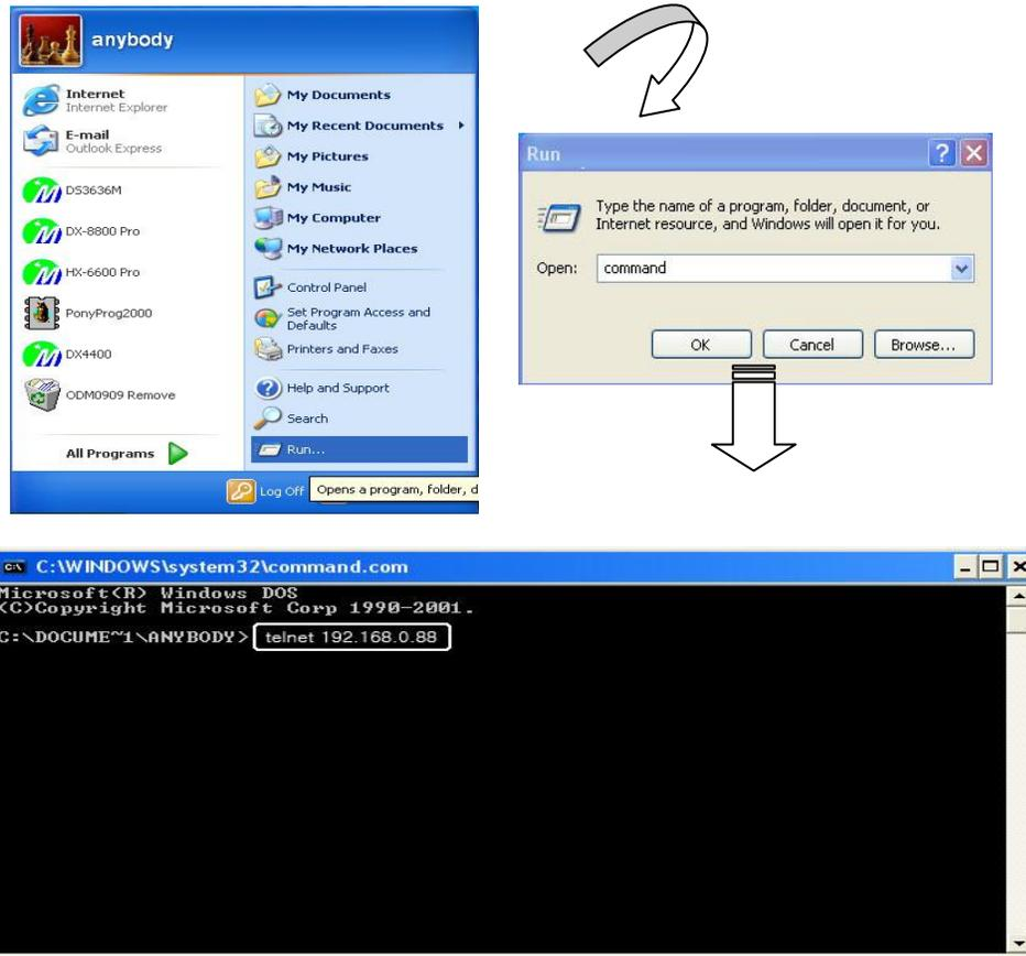
[Fig. 2-5] TELNET window
