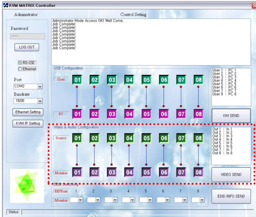
[Fig. 1-4] Video/audio distribution in separation of USB switching in PC program
