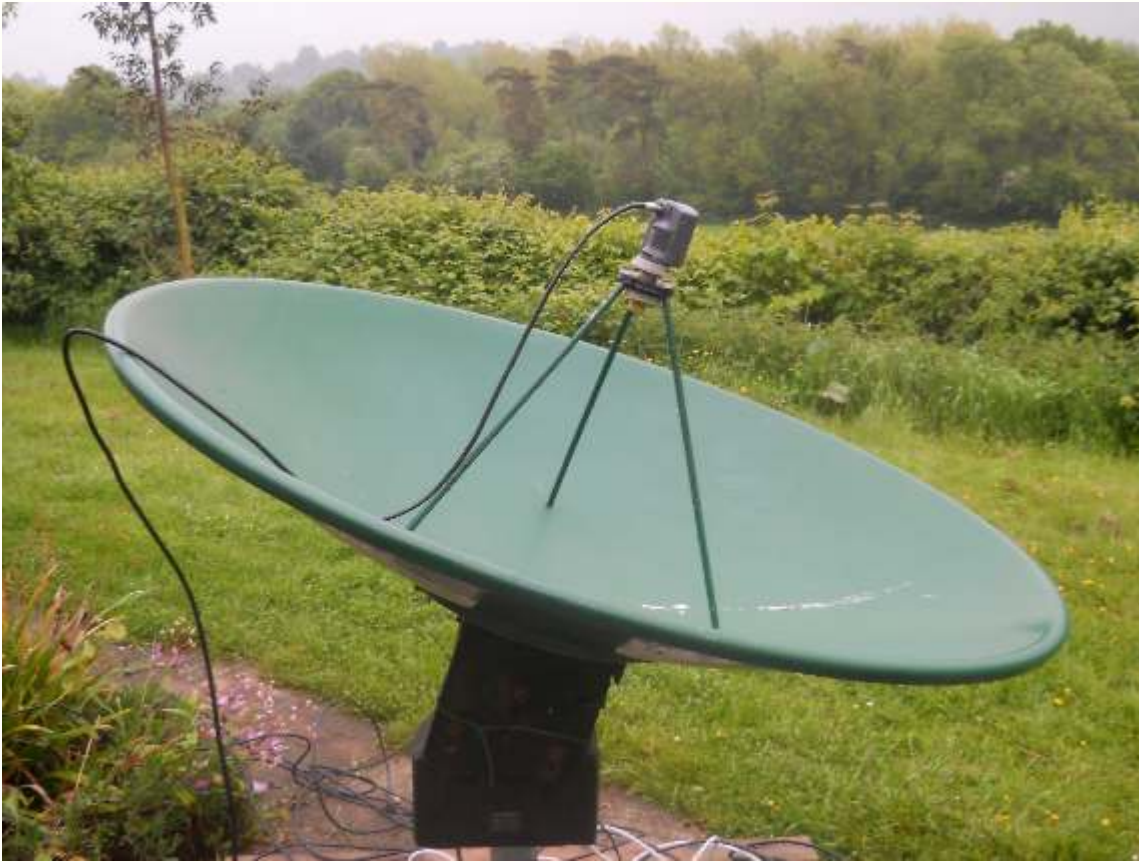
The 1.2m dish with Ku LNB
