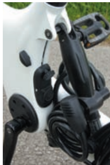
ABOVE AND BELOW: The twin-leg 'display stand' tucks away very neatly against the swingarm when not in use.
