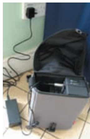
ABOVE: The mains charger is fairly small and light, and fits within the battery bag if necessary. Charge time from empty is around six hours, and you can top up the battery at any time.
