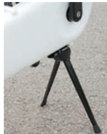
ABOVE AND BELOW: The twin-leg 'display stand' tucks away very neatly against the swingarm when not in use.
