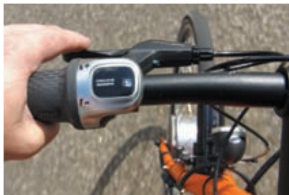
On the pedelec version, the twist-grip throttle (ABOVE LEFT) only adds power when the sensor (ABOVE) detects pedalling. The hub gear shifter (LEFT) is upside down on the left side of the bar.
