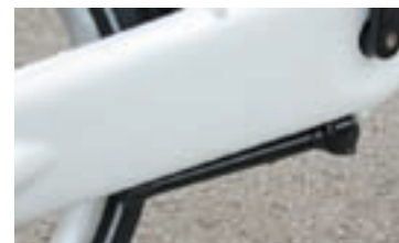
ABOVE AND BELOW: The twin-leg 'display stand' tucks away very neatly against the swingarm when not in use.
