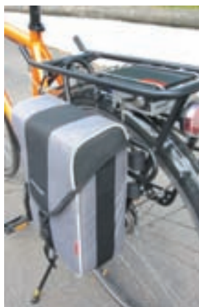
ABOVE LEFT: The battery can be unplugged and detached from the bike for recharging.
