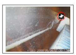
If the system is setup to record streaming videos, the "VIDEO" icon can be seen at the bottom center of the screen in the "Live Video Mode" and the SnakeEye III is ready to record streaming video.
