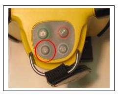
4. Turn on/off and adjust three intensity levels of the light source on the camera head by pressing the "Camera Light Source" button on the operational keypad. Pressing the "Camera Light Source" button will toggle the camera lights through the Low, Medium, and High Intensity and then Off cycle.
