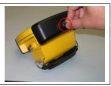
Step 7: Install SD Card Cover & Tighten Screw
