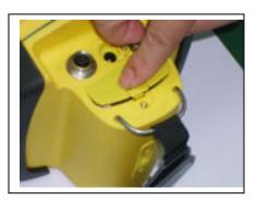
Step 1: Insert a fully-charged battery into the battery compartment.
