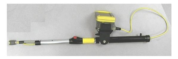
Camera and Display mounting platform to extend the viewing reach of SnakeEye. Each pole has multiple extension locking positions spaced at six-inch intervals. The pole may be rotated within the handle to give 360° viewing. The camera head may be articulated 130° from the straight position.
