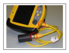
Step 8: Connect cable to Display Unit & Camera Head
