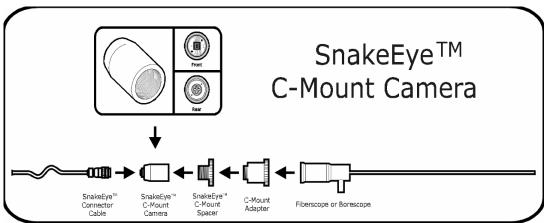
This optional accessory greatly expands the capabilities of the SnakeEye<sup>TM</sup>III Base Kit by adapting to fiberscopes and borescopes, providing visual access to areas as small as 4 mm in diameter.
