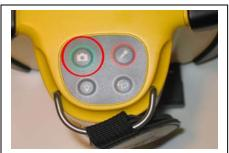
Pressing the "Image Recording" button on the operational keypad, the SnakeEye III will store the "current displayed image" onto the SD card after first checking for available space on the SD card. The user will briefly see the recording symbol and the amount of space available on the SD card at the right-top corner of the display screen.
