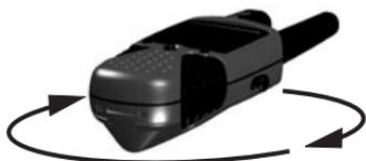
*Calibrating the compass: Hold the unit level and face up. Turn the unit around as shown above.*
