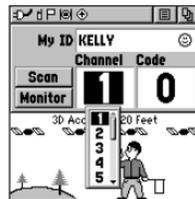
Select from FRS 1–14, GMRS 15–22 (with GMRS enabled), and 15R–22R GMRS repeater channels (with GMRS and Repeater Channels enabled).
