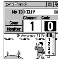
*Choose from 38 squelch codes. Setting the unit to zero will allow you to hear all transmissions on that channel, but you must be on the same squelch code to radio back.*
