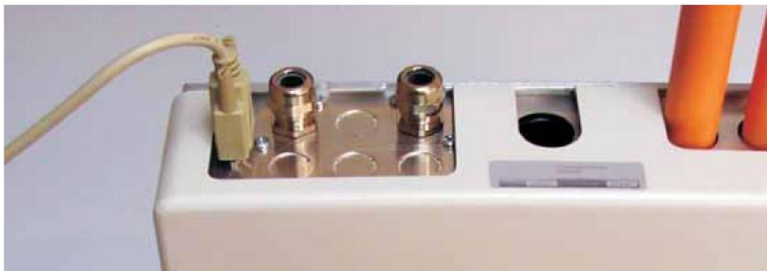
Figure 26: Connecting a PC to the command module's RS-232 port
