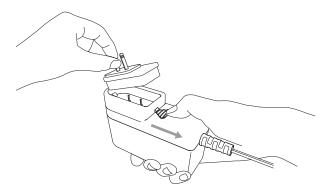
2 Release latch when the plug adaptor locks in place.
