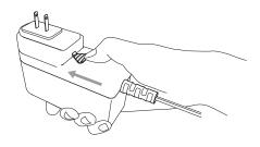
To disassemble, push latch outward to remove or replace plug.
