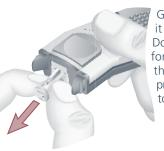
Grasp the lancet body and pull it straight out of the device. Do not reuse lancets, they are for single use only. Dispose of the used lancet carefully to prevent injury or contamination to others.
