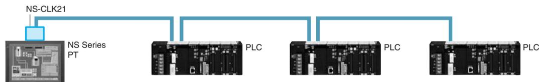
If a Controller Link connection is used, data links can be set between PLCs and multiple PLCs can be monitored/set from the NS-series PT's screen.
