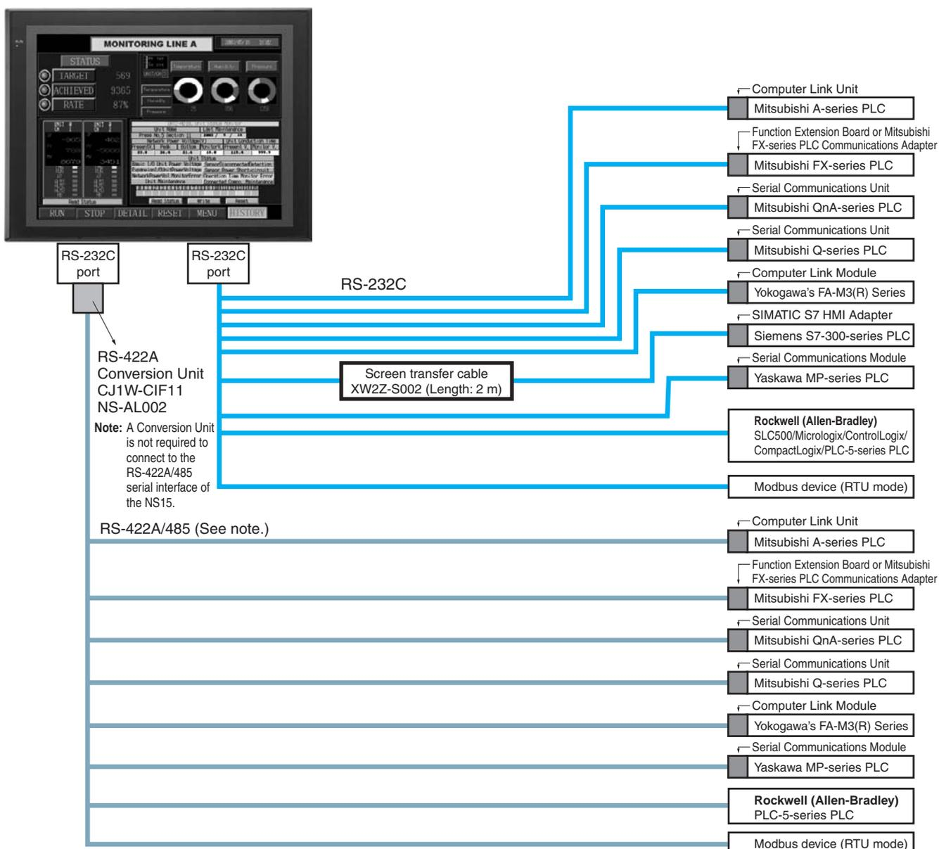
Note: Whether an RS-422A or RS-485 connection is supported depends on the device that you are connecting to. For details, refer to the Connectable Devices page or NS-Series Programmable Terminals HOST CONNECTION MANUAL Multivendor Connection (Cat.V092).
