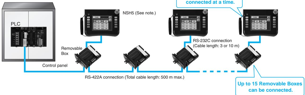
**Note:** Before removing the NSH5 from the Removable Box, be sure to first turn OFF the power supply key on the Removable Box.
