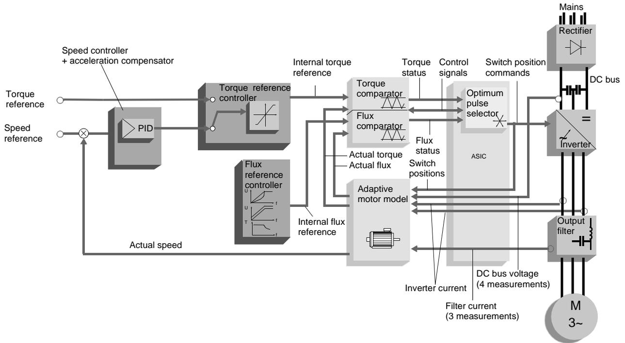
*How does DTC Differ from PWM Flux Vector Drives?*
