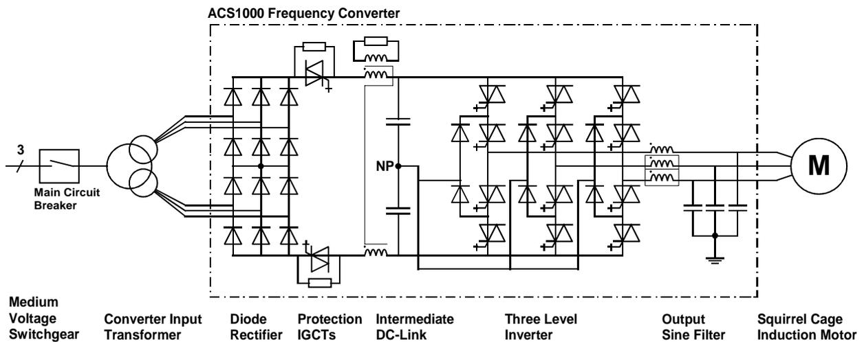
Each leg of the 3-phase inverter bridge consists of a combination of 2 IGCT's for 3-level switching operation: with the IGCT's the output is switched between positive DC voltage, neutral point (NP) and negative DC voltage. Hence both the output voltage and the frequency can be controlled continuously from zero to maximum, using Direct Torque Control.
