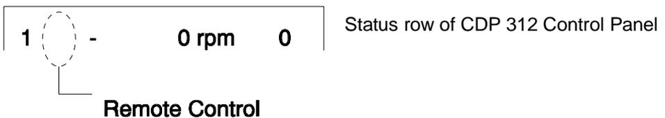
**Local Control** If the converter is switched to local control, local operation from the push-button on the converter front door and from the CDP 312 control panel is possible. In local operation mode no remote control command will be accepted.
