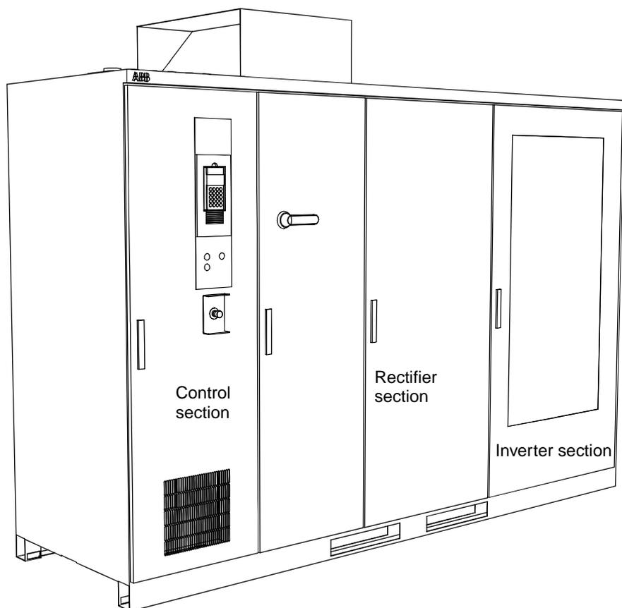
**Cabinet Sections** The ACS 1000 is designed with the inverter unit as one complete section including output filter capacitors and DC link capacitor. This section, located on the right hand side, experiences maximum air flow which is advantageous for the temperature sensitive capacitors. Construction allows easy exchange of IGBT's using a special tool.
