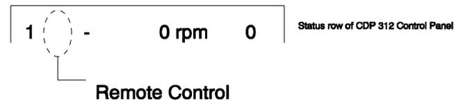
***Local Control*** If the converter is switched to local, local operation from the pushbuttons on the converter front door and from the CDP 312 control panel is enabled. In local operation mode no remote control command will be accepted.
