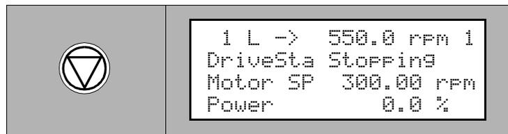
The unit stops following the preset stop function. The main circuit breaker remains closed.
