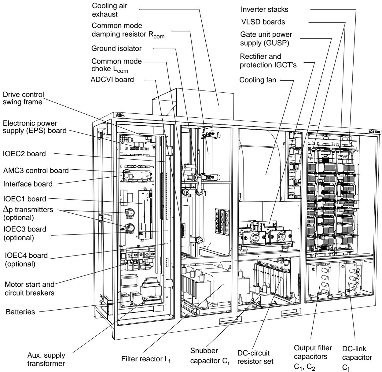
Behind the swing frame and a protective separation door is the drive's power terminal section. To provide adequate access to this section, the swing frame can be opened through more than 90°.
