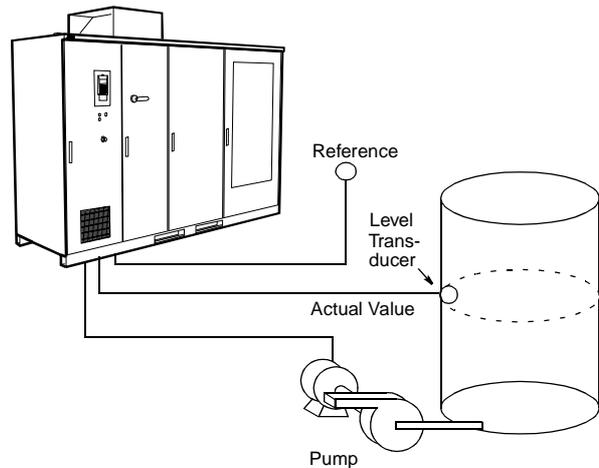
The internal PID controller of the ACS 1000 eliminates the need to provide, mount, and wire a separate PID controller.
