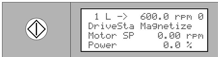
After a few seconds the motor is driven up to reference speed following a preset ramp.
