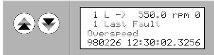
**Actual Signal Display** Actual signals are used to monitor ACS 1000 functions and do not affect the performance of the drive. Actual signal values are measured or calculated internally and they cannot be set or altered by the user.
