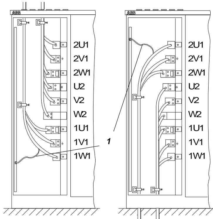
Cable lead through from top      Cable lead through from below
