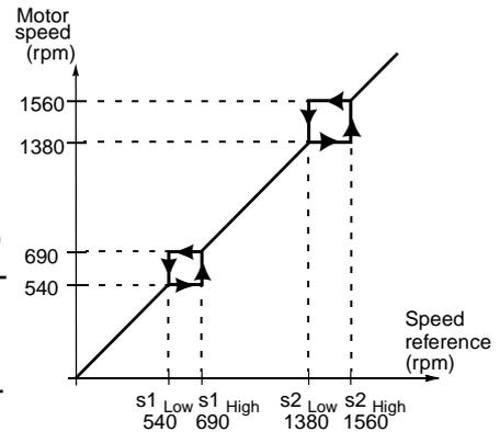
Critical speed areas are set with parameter group 34, *Critical Speed*. For further details see *Appendix K - Signal and Parameter Table*.
