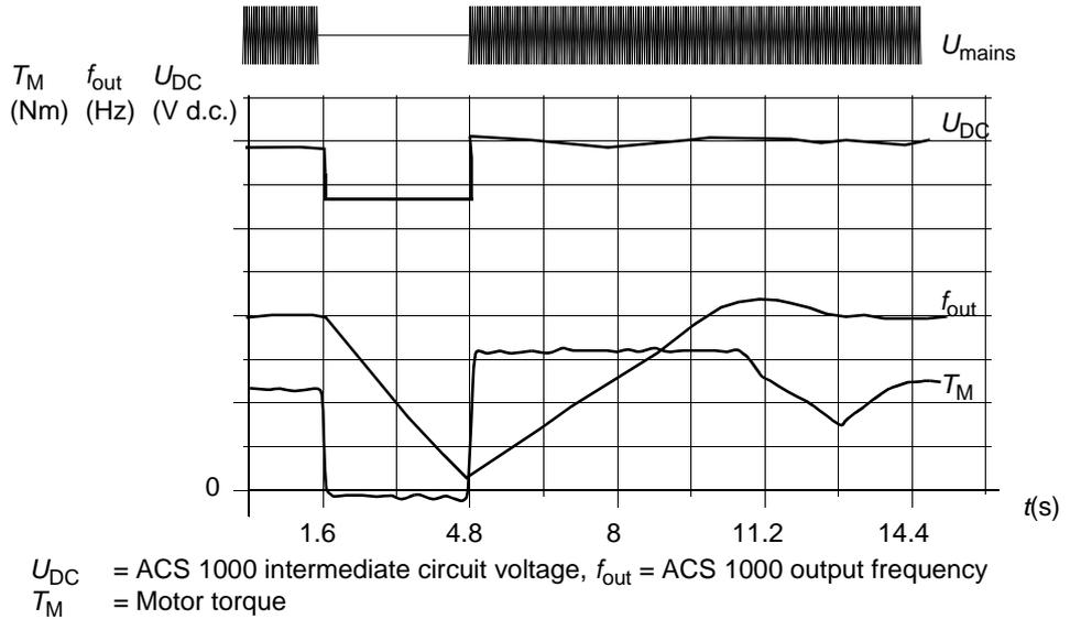
The intermediate circuit DC voltage drops to the minimum limit. The controller keeps the voltage steady as long as the main power is absent. The ACS 1000 runs the motor in generator mode. The motor speed falls but the drive is fully active as long as the motor has enough kinetic energy.
