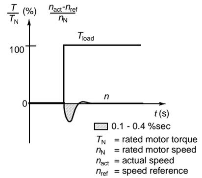
Table 3-1 Typical performance figures for speed control, when Direct Torque Control is used.
