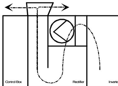
From the front door intake, the air flows through the heat sinks of the vertical inverter stacks and is then routed to the central section where the fan is located. After passing the fan, the air is blown through the rectifier diode stacks, followed by the motor filter reactor. The exhaust is located on top of the cabinet and provides a natural stack effect in order to direct the air flow after the fan. The exhaust is covered in order to protect the equipment inside mechanically.
