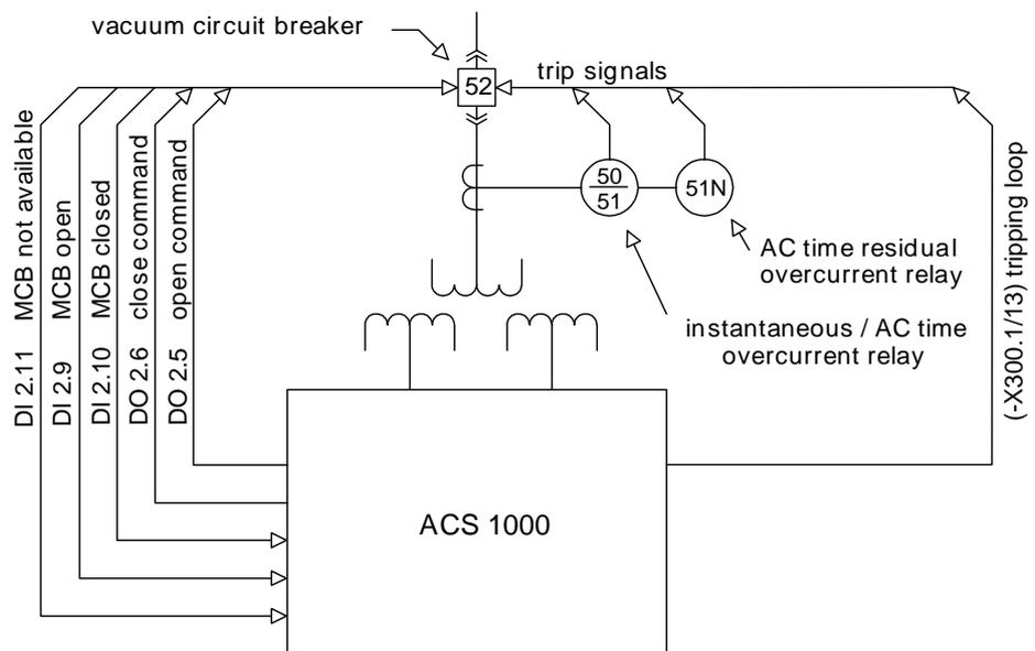
Figure 10-3 Mains connection scheme with vacuum controller
