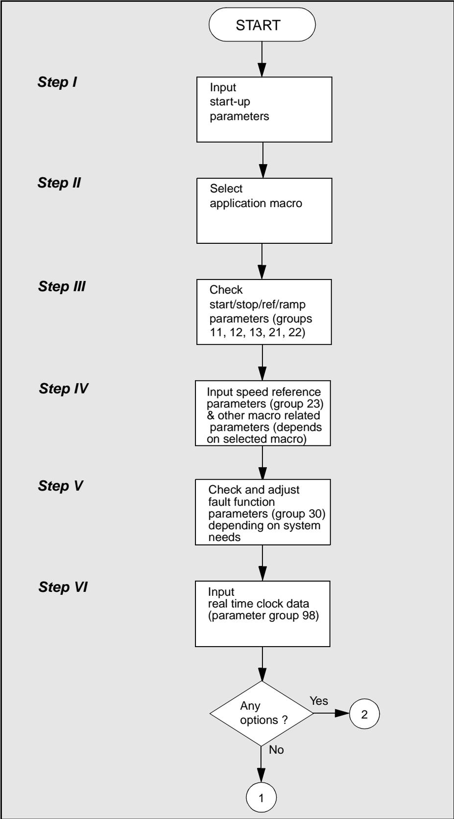
Figure 6-1 Application parameter programming procedure (continued)
