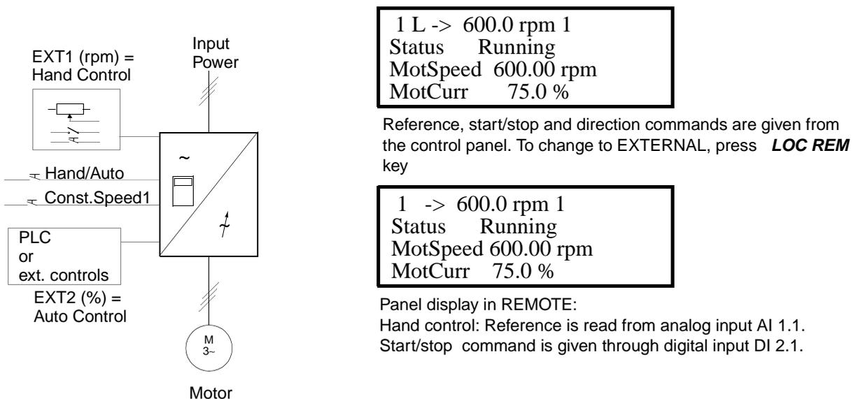
*Input and Output Signals* The default I/O signals of the Hand/Auto Macro regarding opening/closing the MCB, starting/stopping the drive, speed, control location, reference and actual values are shown in the following table. The corresponding parameters are listed as well. For further settings refer to *Appendix K - Signal and Parameter Table*.
