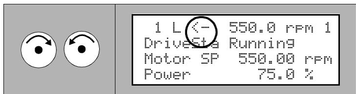
If the motor is running, the speed will automatically ramp to zero and the motor will reverse its sense of rotation and resume preset speed.
