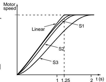
Acceleration and deceleration ramps are set with parameter group 22, *Ramp Functions*. For further details see *Appendix K - Signal and Parameter Table*.
