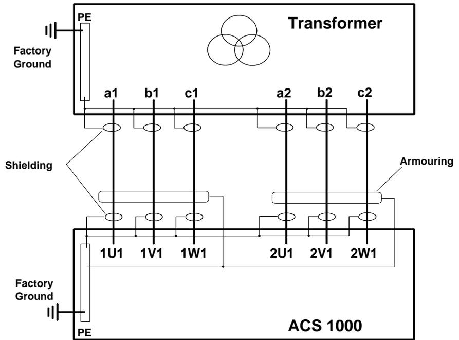
Figure 10-6 shows a typical motor cable connection. The actually applied connecting scheme must comply with local regulations.
