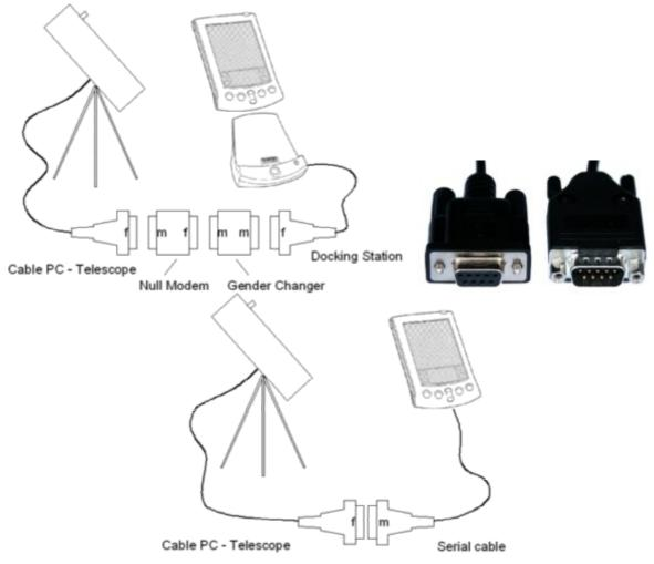
The null modem crosses the serial data lines, so that the telescope and the handheld do not both talk on the same line while listening on the other.
