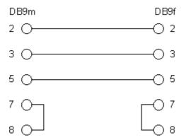
In this wiring diagram I put the bridge on both sides, so it will work with any setup, but in fact you will need it only on the Palm side. Put this adapter just after the Palm cable, before any null modem or gender changer.
