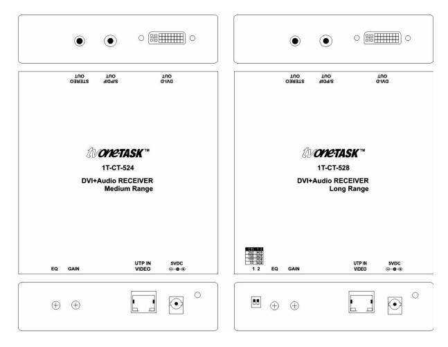
Note: If the CAT.5/Cat.6 cables runs are equal to or less than 100 Meters (325 Feet), you can use either the 1T-CT-524 or 1T-CT-528 Receiver to complete the system. If the cable runs are between 100 Meters (325 Feet) and 250 Meters (800 Feet), you must use the 1T-CT-528 Receiver.
