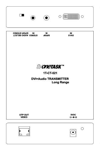
Connect the DVI-D source device's output to the DVI-I IN connector of the 1T-CT-521 Transmitter, using the appropriate DVI cable. Then connect either an S/PDIF audio signal or an analog Stereo audio signal to the appropriate connector.
