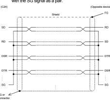
3) Do not connect an RS-422 device to the RS-232C interface. If an RS-422 device is connected to the RS-232C interface, the RS-422 interface hardware for the connected device will be damaged and communications cannot be performed.
