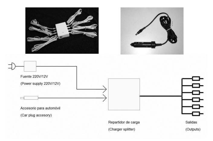
Plug the car plug accessory or another power supply on the splitter inlet. The power supply must have the following specification:
