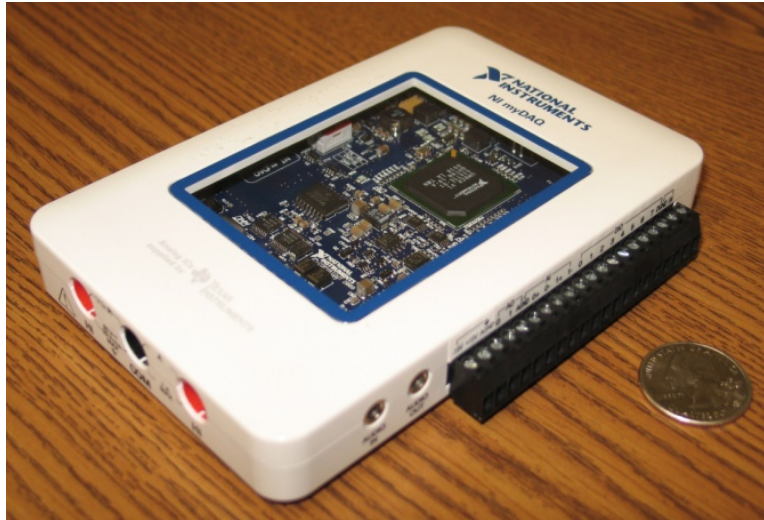
Figure 2. National Instruments myDAQ® personal instrumentation platform. 10
