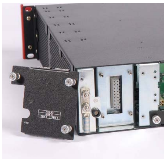
Figure 15 - Shelf ID Board with two E 2 PROMs (rear cover removed).
