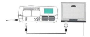
Before setting-up, switch off all equipment. The projector may be connected a 1080p 50-60Hz image source only using DVI-D (Digital Visual Interface).
