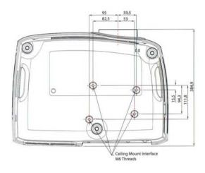
The projector can be ceiling mounted using an approved UL tested/ listed ceiling mount fixture, with a capacity of minimum 60 kg / 130 lbs.
