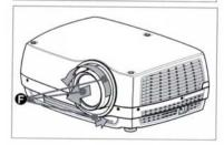
A range of fixed and zoom lenses is available to cover most applications, both front and rear. The lenses are powered and fitted with a bayonet mount for ease of installation.
