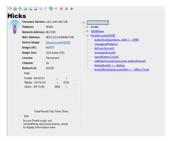
There are four network configuration parameters: Network Address, MAC Address, Channel, and Network ID.
