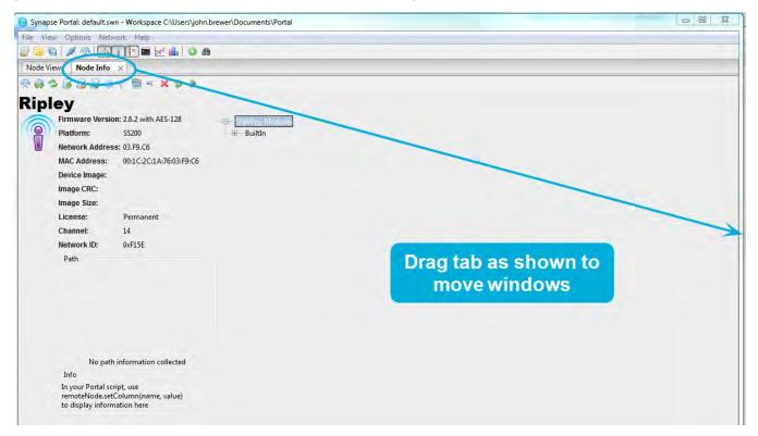
Window panes may be resized by clicking and dragging the horizontal and vertical borders separating them. If you have made changes to your window placement and sizing and wish to have **Portal** return to its default layout, select **View** - **Rearrange to Default View** and you will be returned to a view with the **Node Views** window on the left, the **Node Info** window on the right, and the **Event Log** window across the bottom of the screen.
