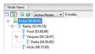
In this example network we can see that node 03.E8.99 routes packets through the bridge node, 03.F9.C6, to reach **Portal**, while node 04.00.9D is routed through node 04:CB.47 to reach **Portal**. As nodes are spread apart and it is necessary for nodes to "hop" through other nodes, the tree view can become more and more branched. This view enables you to see a snapshot of how nodes route messages through each other through the **SNAP** mesh network.
