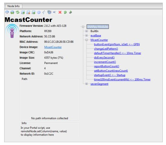
The **BuiltIn** functions represent the core **SNAPpy** feature set, and are functions that can be called from **Portal** even when no user script has been uploaded into the node. These same functions are also always available for use *within* scripts.
