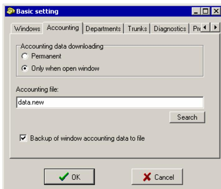
The data can be uploaded either continuously (during the whole program run) or whenever one accounting data window at least is displayed on the screen. All accounting data are uploaded from the PBX into a selected accounting file used for accounting data processing. Selecting the **Accounting Window Data Saving into File** item you load a certain number of accounting lines from the file upon the start of the application.
