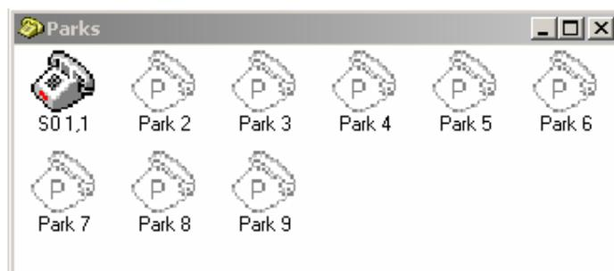
The 2N<sup>®</sup> - OMEGA Lite PBX is equipped with nine parking places. And this window displays the status of each parking place separately.
