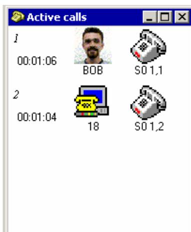
The call line shows information on the bus used for the call, call duration, and list of calling lines. The lines are sorted according to calling lines. *Subscriber line* icons are displayed *at rest* as taken over from the subscriber line window.
