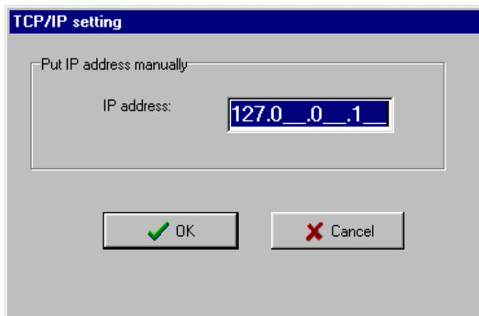
It is a target address of OMEGA - AGENT that provides contact with the 2N<sup>®</sup> - OMEGA Lite PBX.
