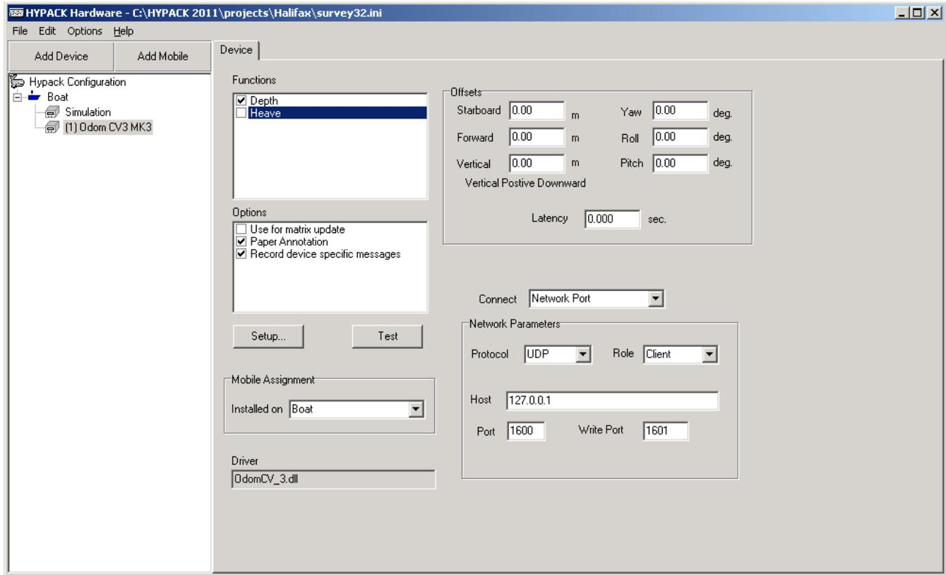
Next click on the Setup... button but make sure the Hydrotrac device is highlighted under the Hypack Configuration menu. Make sure Channel 1 under the setup menu is set to Bathy and all other channels are turned Off.
