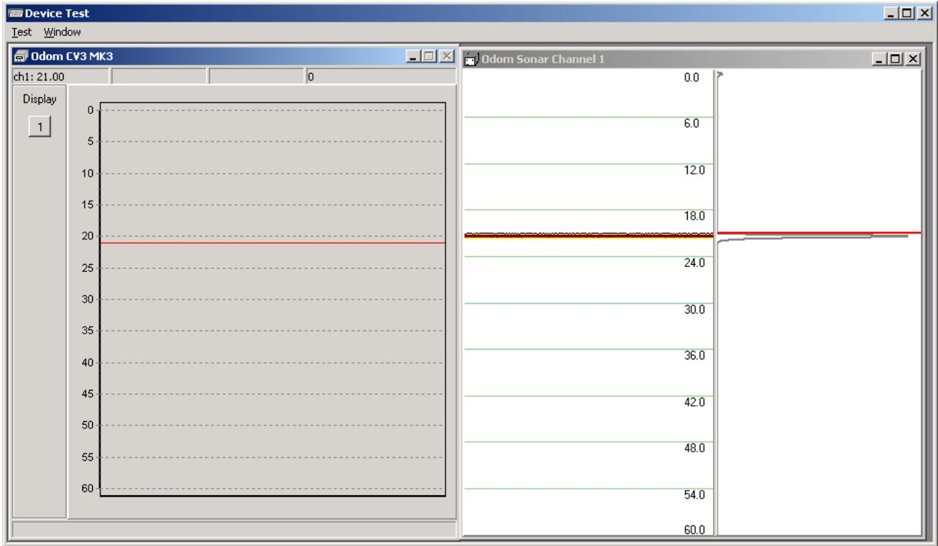
Initially when starting the test only the window labeled Hydrotrac will open up. Click on the 1 button to display the signal from channel. Click anywhere on the Odom Sonar Channel 1 window and select beam to display the actual signal. Once the data is verified close the window and start Hypack survey.
