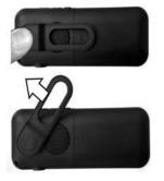
If the belt clip is installed, you must lift it up and maintain it in this position during the battery installation or replacement. You can also turn the belt clip counterclockwise.
