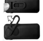
If the belt clip is installed, you must lift it up and maintain it in this position during the battery installation or replacement. You can also turn the belt clip counterclockwise.
